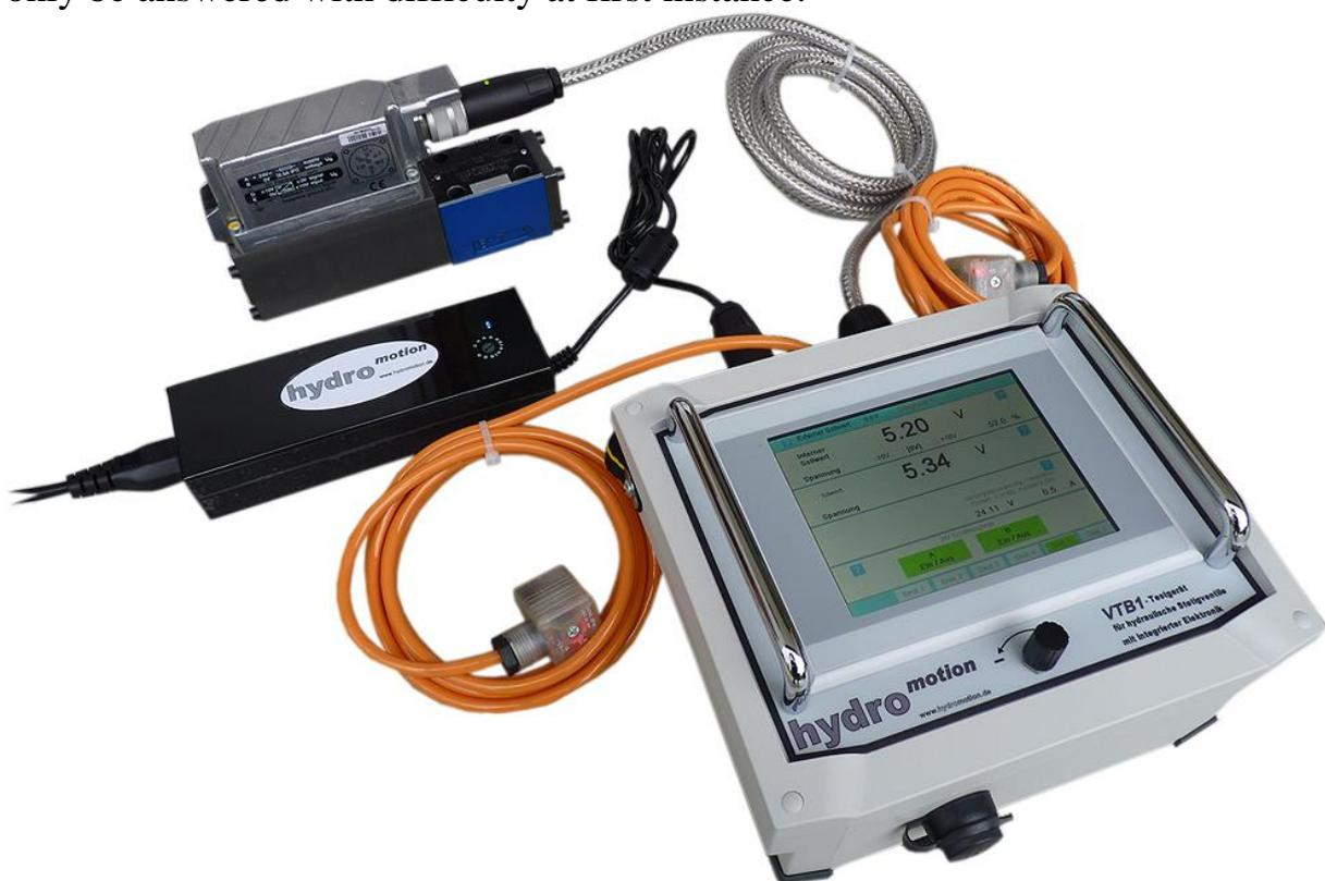
With modern hydraulic valves with integrated electronics (**On Board Electronics**) the electric signal cable is connected to the valve directly, without further measurement sockets or optical feedback.
